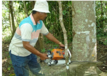
Figure 1. Making notch fall by the operator
